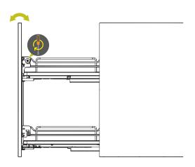
Loosen the 3.9x13 screws, to adjust the door to the right and left and insert the four covers as shown.
