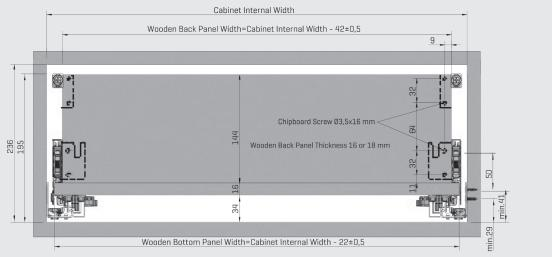
Calculation Method for Front Panel Dimensions:Cut Measurement=Cabinet Internal Width - 124 Calculation Method for Front Gallery Railing Dimensions:Cut Measurement=Cabinet Internal Width - 57
