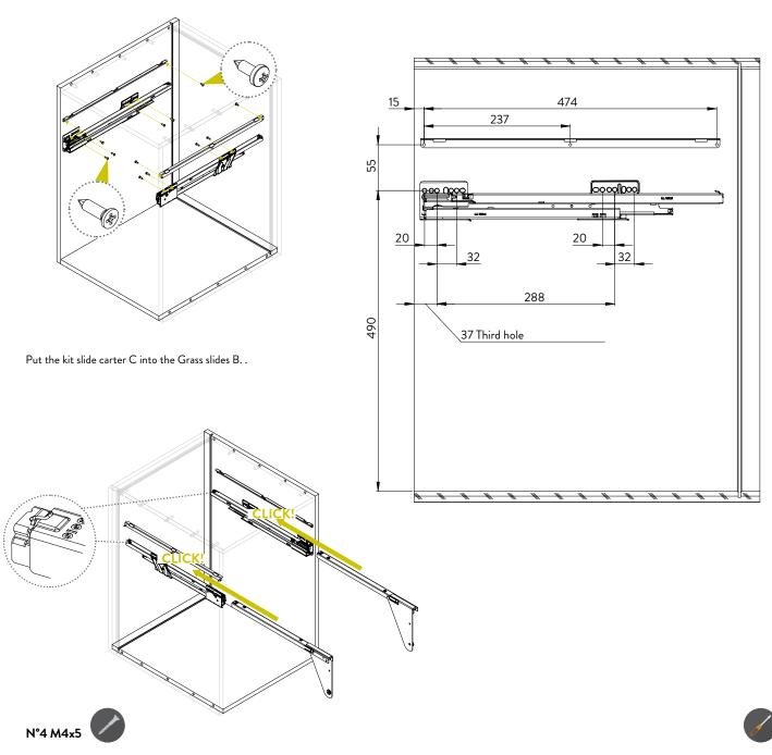
Screw the metal box A into the kit slide carter C by using the specific provided screws.
