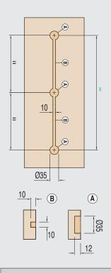
X = 2240mm outer bore centre distance for shorter doors simply cut threaded rods.
