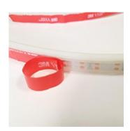
Peel back the remaining red tape and install the LED strip as desired.
