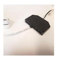
Plug the power lead into the connector block on the LED driver.
