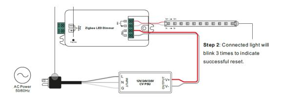
**Note:** 1) If the device is already at factory default setting, there is no indication when factory reset again. 2) All configuration parameters will be reset after the device is reset or removed from the network.
